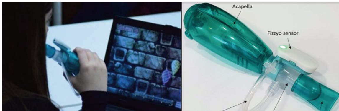
Figure 1: Fizzyo sensor attached to an Acapella OPEP being used to play a game (left) and as a labelled diagram (right). The sensor can also be attached to other common devices (not shown).
