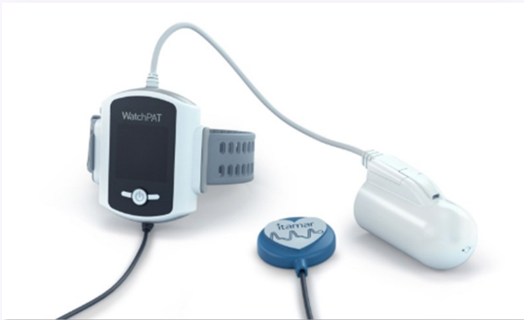
Figure 2: The WatchPAT 300 device showing the main unit that fits around the patient's wrist, the novel PAT finger probe, and the optional snore / body position sensor (Itamar Medical Online 2021 – image used with permission)
