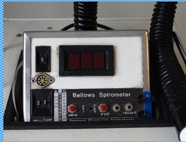
Spirometer display showing tumblers for program setting (upper one), setting the time interval for the FEV (lower left hand) and BTPS temperature correction (lower right hand). The socket below the upper tumbler links to an XY plotter to print the flow-volume curve in delayed time. The jack plug socket marked 'record' provides an output to the cassette recorder.
