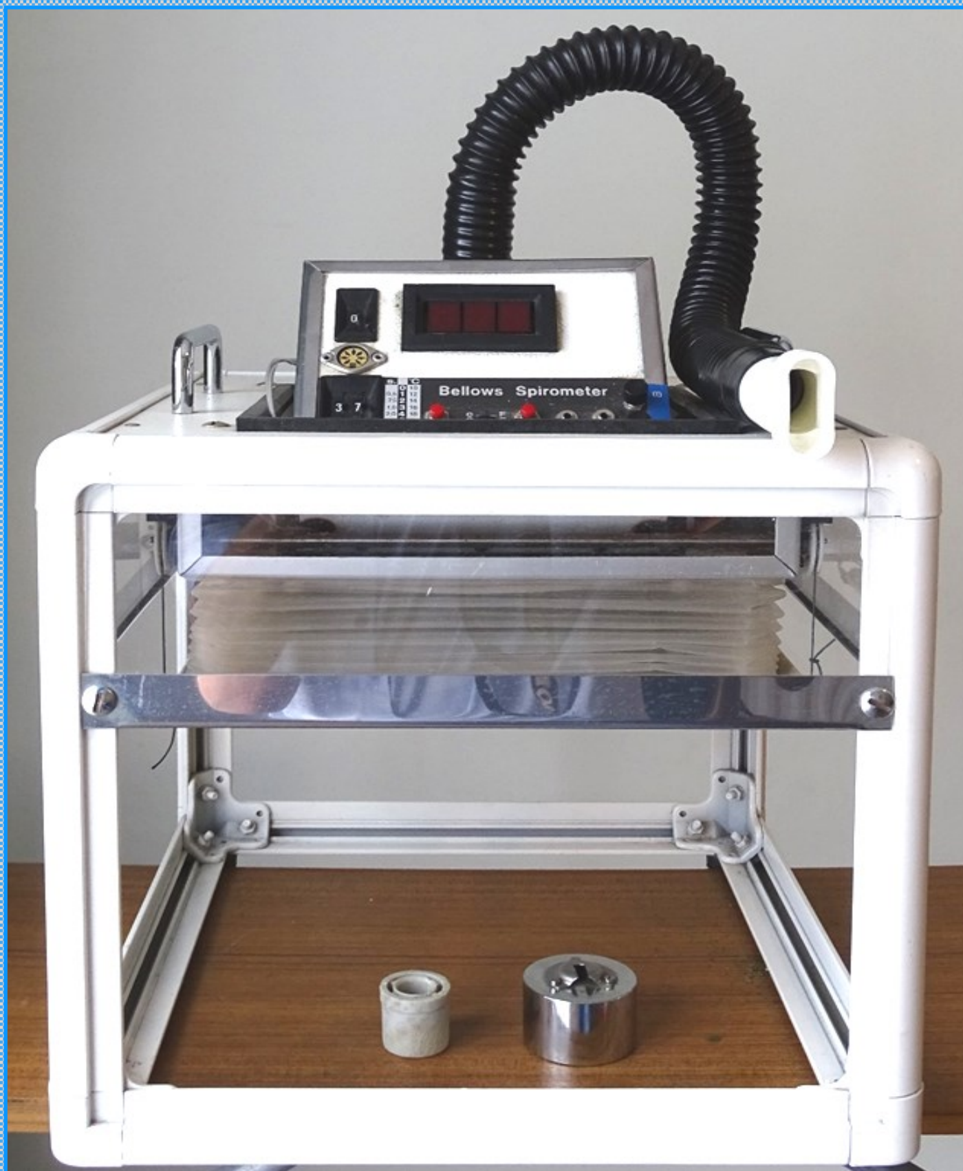
McDermott, dry bellows, digital spirometer with calibrating weight and orifice, 1980 Garw Electronic Instruments, Glamorgan, South Wales
