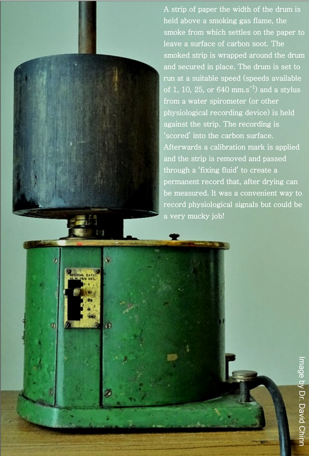
Sherrington Stirling Kymograph Recording Drum (C F Palmer (London) Ltd), c. 1955
