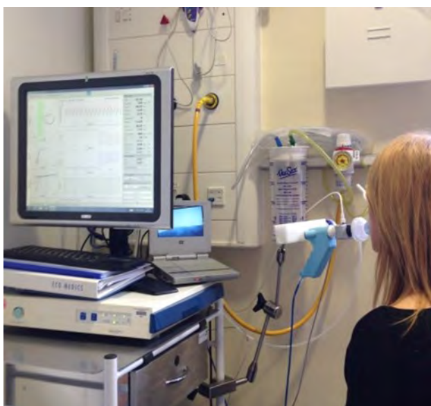
Figure 1 – Participant breathing 100% oxygen for a Nitrogen MBW using the Exhalyzer D (Ecomedics, AG, Switzerland).
