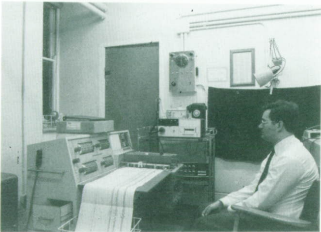
Fig. 2. Investigation room: The patient's room is behind the blackout curtain. Leads from the ear oximeter, 'Respitrace' and other transducers enter through the wall. Data is being monitored on a 16 channel recorder.
